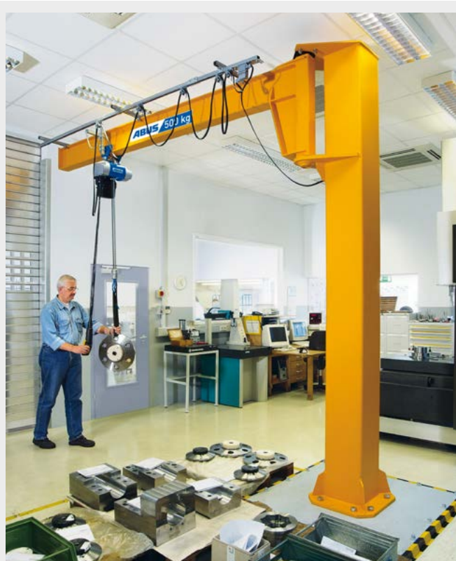
Wall jib crane LWX with electric chain hoist ABUCompact GMC
