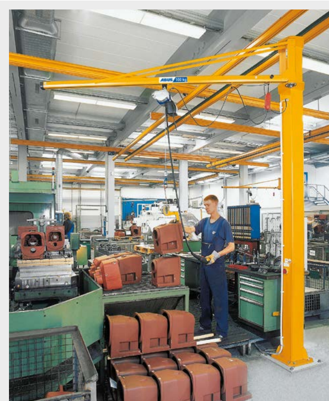
Wall jib crane LW with electric chain hoist ABUCompact GM2
