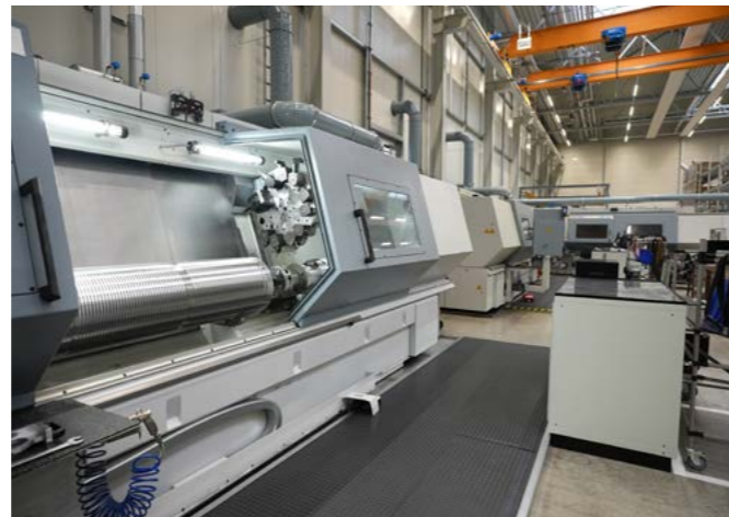
Advanced CNC lathes are used to turn the rope drums in one operation, an approach that ensures perfectly smooth running of the rope drums during operation.
