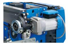
The modular wire rope hoist is driven by a trolley travel motor operated with a frequency converter. The hoist drive has a 4-pole hoist motor with frequency converter control as standard. The lifting speed can be either infinitely adjustable or used to simulate pole switching. The maximum lifting speed is load-dependent and achieves double the nominal lifting
